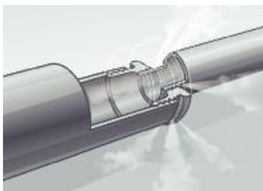
PRODORAL®R 6-1 for leaky thread connections in interior gas pipes
